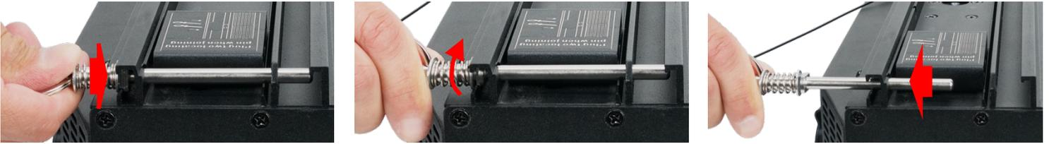
1. Remove spring-loaded locking-pin, compress the spring enough to clear the rail, rotate ring to vertical orientation (stepped rail-block to a horizontal orientation), and pull it straight out.
