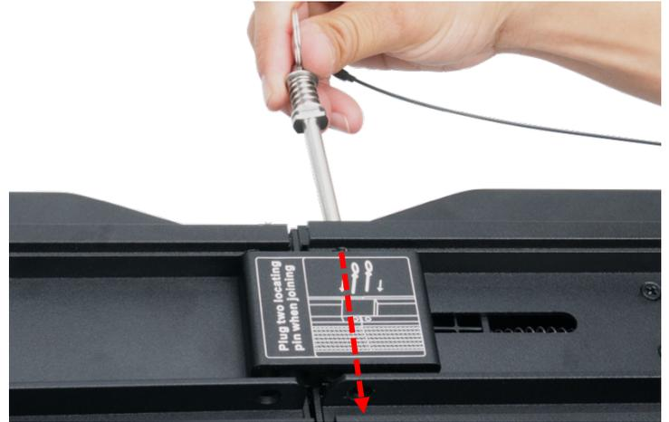
4. With both fixtures horizontally adjoined, align the locking-pin rail holes with the holes in the locking-pin abutment-block, and insert one locking-pin into the first set of aligned holes.
