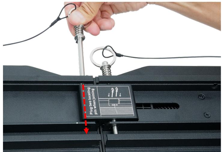
5. Compress the spring of the first locking-pin and rotate the ring 90° to lock it into the rail. Insert and lock a second locking-pin through the second set of aligned holes and ensure that the stepped rail-block of the locking-pin is horizontally aligned with rail slot to pass it through rail slot.
