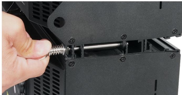
2. With the locking-pin rail holes aligned, insert a locking-pin at each end (compress the spring of the locking-pin and rotate the ring 90° to lock it into the rail).
